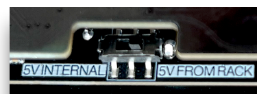
5 V selector switch on the rear side of the module
